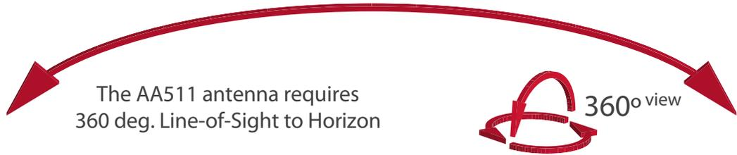
The bottom of the antenna must be at least 0.15m (.5ft) above building
